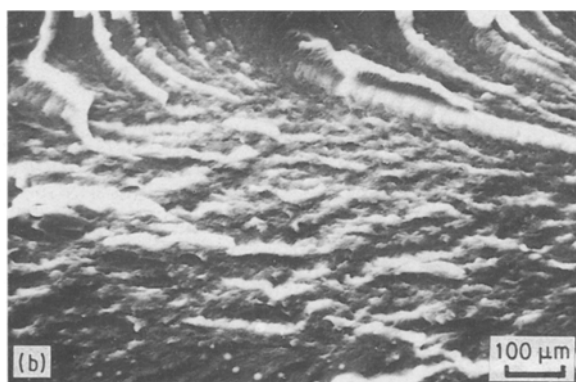
Figure 4 Scanning electron micrographs of the fracture surface of material C: (a) the whole fracture surface; (b) higher magnification.
