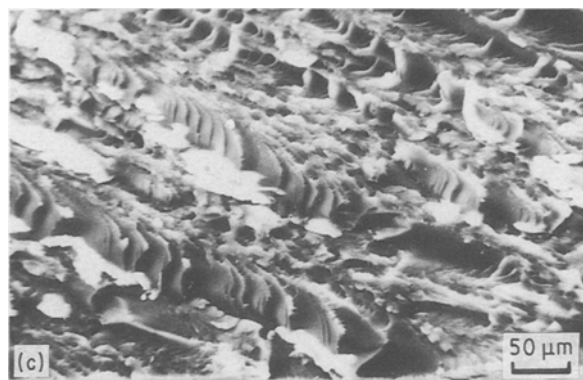
Figure 3 Scanning electron micrographs of the fracture surface of material B: (a) the whole fracture surface; (b and c) higher magnifications of two parts of the rough region.
